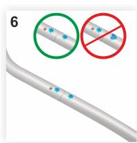
4-6. Applying the same method mentioned above, add the corner items to the curved bars making sure to match the numbering / marking from the elements that merge, as in Figures 5-6.
