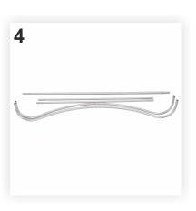
3. Join all the aluminum bars from the package provided with elastic until you will get: two straight bars (for the vertical sides), two curved bars (for the horizontal sides) and one support stick.
